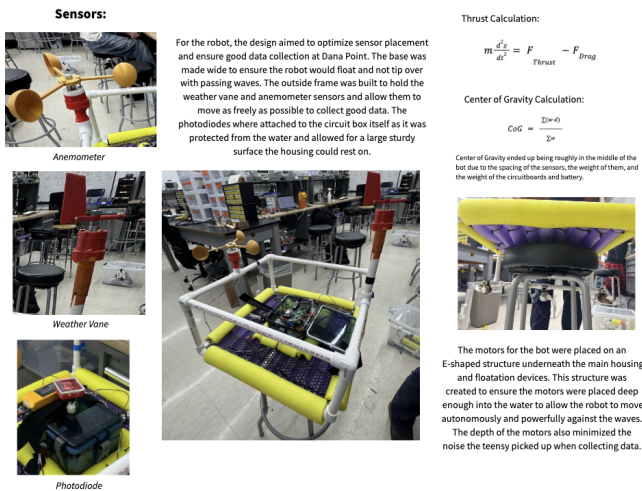
Fig. 4. Mechanical design and integration of the surface vehicle. Sensor placement labeled (anemometer on the upright mast, weather vane on the opposite mast, photodiode mounted flat on the electronics enclosure). Bottom panels show the E-shaped underwater motor mount that places the motors deep enough to drive the vehicle through chop while keeping the motor electrical noise away from the magnetometer above the deck.
